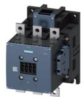
power contactor, AC-3e/AC-3 300 A, 160 kW / 400 V, AC (50-60 Hz) / DC Uc: 220-240 V 3-pole, auxiliary contacts 2 NO + 2 NC drive: conventional main circuit: busbar control and auxiliary circuit: screw terminal
